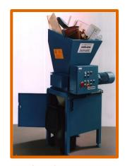
**Note:** The blades can be used in various widths. This allows you to determine the dimensions of the final product yourself. Installation is exclusive of collection container. The B400 frame is suitable for 120 L containers and the B600 frame is suitable for 240 L containers.
