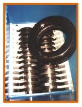
**Note:** The blades can be used in various widths. This allows you to determine the dimensions of the final product yourself. Installation is exclusive of receiving container and shuttle.
